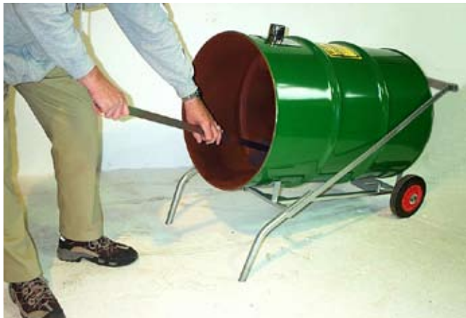
b) Scrape the heavy load out of the Big Brute.
